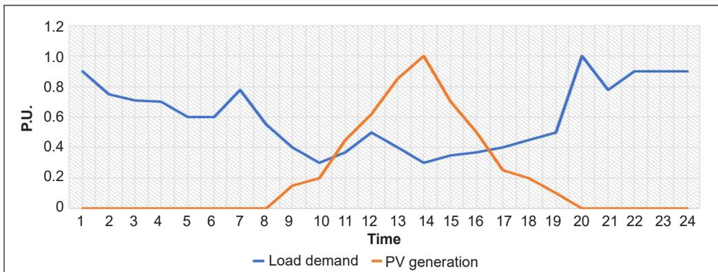
Figure 3. PV generation and load demand profile
