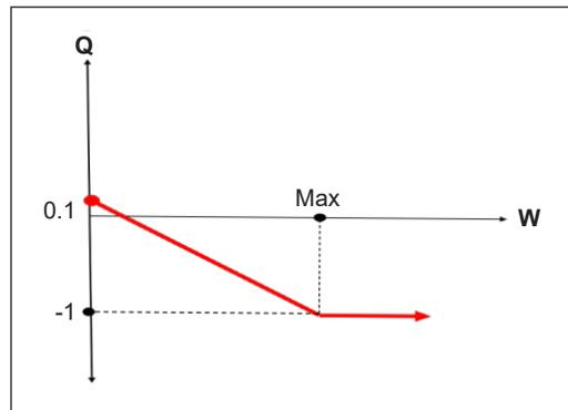
Figure 4. Proposed technique response to PV active power injection
