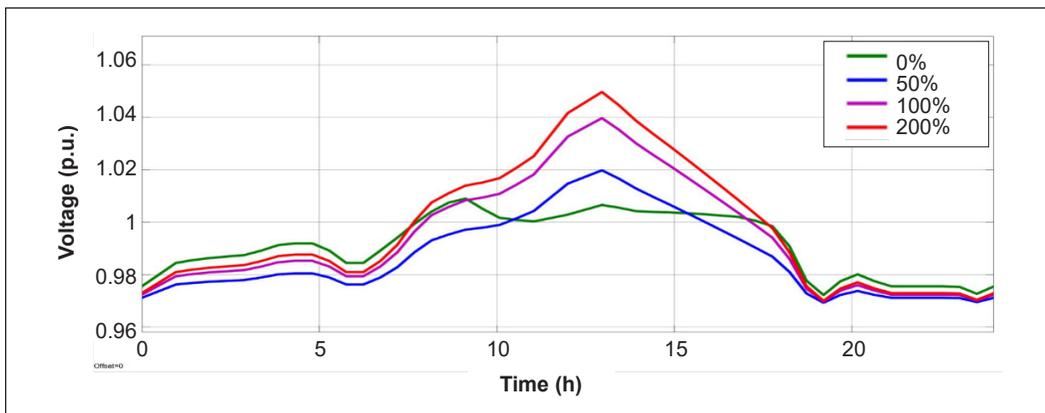
Figure 11. The voltage graph on the point of common coupling of the last customer on Feeder 3 for 24 hours with the proposal reactive power control for a different level of penetration (0%, 50%, 100%, 200%)
