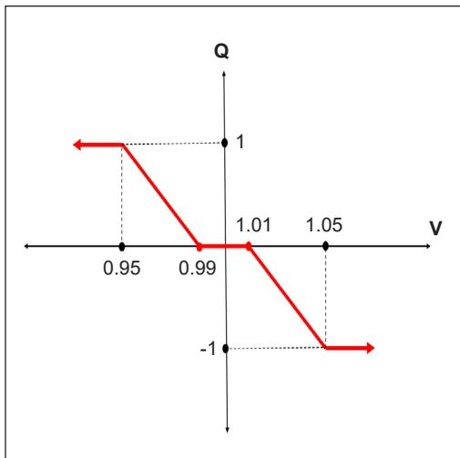
Figure 5. Proposed technique response to the voltage on the point of common coupling
