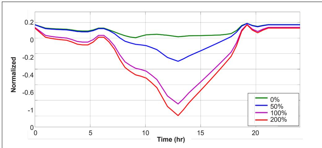
Figure 12. Reactive power injection of the proposal reactive power control for the last customer on Feeder 3 during 24 hours for different level of penetration (0%, 50%, 100%, 200%)
