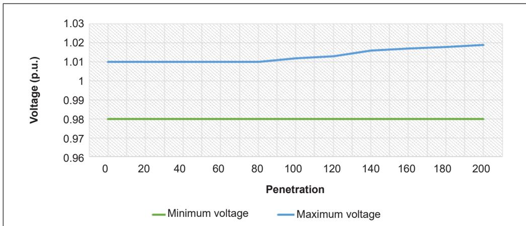
Figure 10. The highest and lowest voltage of the distribution network for different levels of PV penetration with the proposal reactive power control
