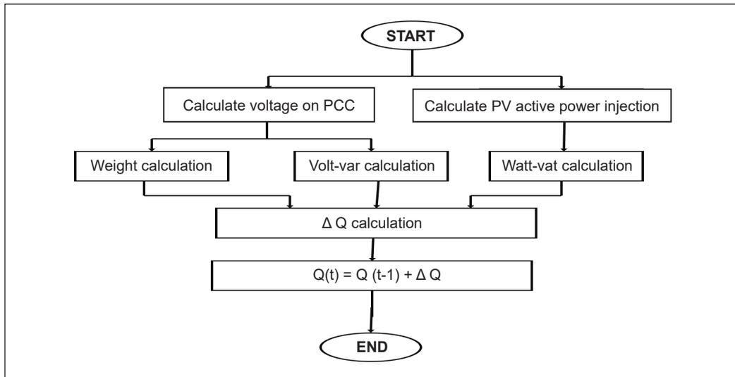
Figure 7. Proposed reactive power control technique flow chart
