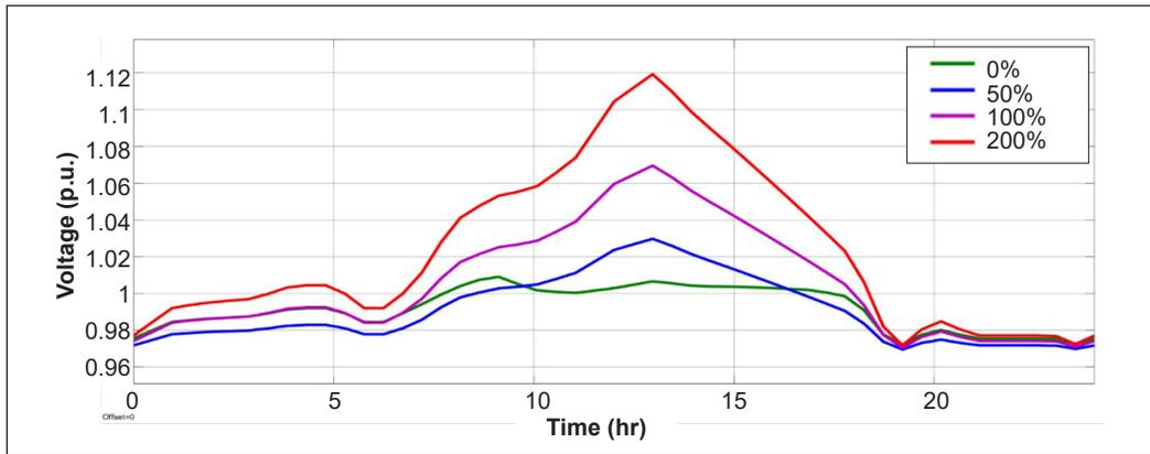
Figure 8. The voltage graph on the point of common coupling of the last customer on Feeder 3 for 24 h without reactive power control for a different level of penetration (0%, 50%, 100%, and 200%)
