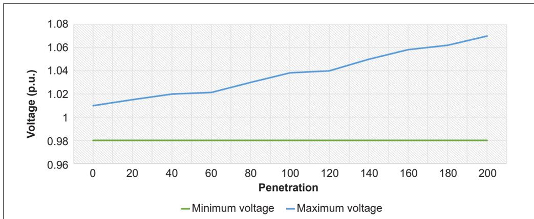
Figure 9. Highest and lowest voltage of distribution network for different levels of PV penetration without reactive power control
